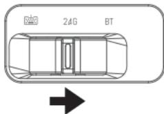
3. Turn the mode rotary knob to 2.4G mode, the Num Lock indicator flashes twice and then goes off, the connection is successfully completed.
