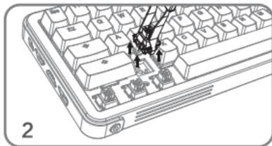
2 Pull out the switch with a switch puller.
