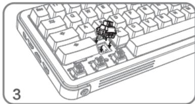
3 Check the installation position of the switch to be replaced and align the hole positions.
