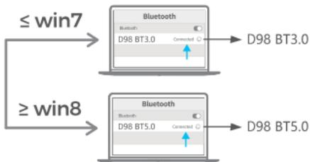
3. Turn on the Bluetooth of your computer or other device, search and select "D98 BT3.0" or "D98 BT5.0" and start Bluetooth pairing until the connection is completed.
