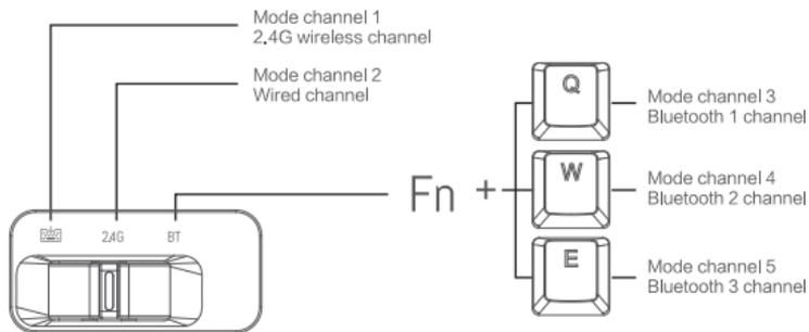
1. Mode channel: The keyboard has 5 channels, BT1, BT2, BT3, 2.4G, wired, and 5 devices can be connected at the same time.
