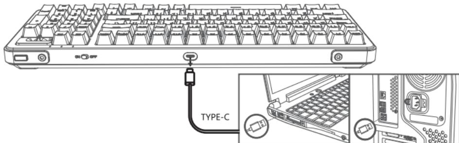
1. Insert the TYPE-C interface of the charging cable into the keyboard, and connect the USB interface to your computer.
