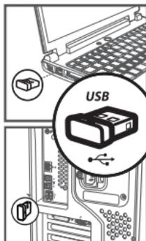
2. Take out the receiver and insert the receiver into the USB port of the computer.
