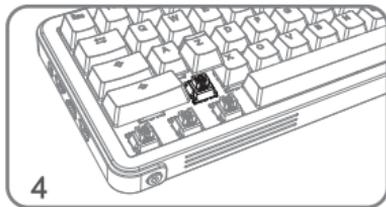
4 Place the new switch on the slot.
