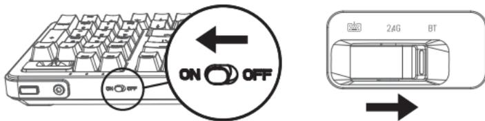
1. Turn the power switch to ON. Turn the mode rotary knob to BT mode, the Num Lock indicator flashes three times and then goes out.
