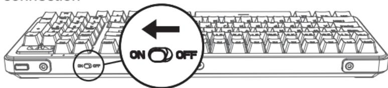
1. Turn the power switch to ON.
