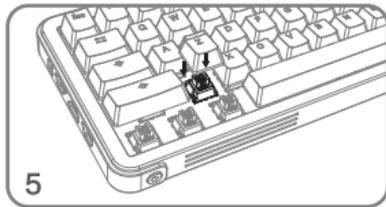
5 Gently press the new switch to install it into the slot.
