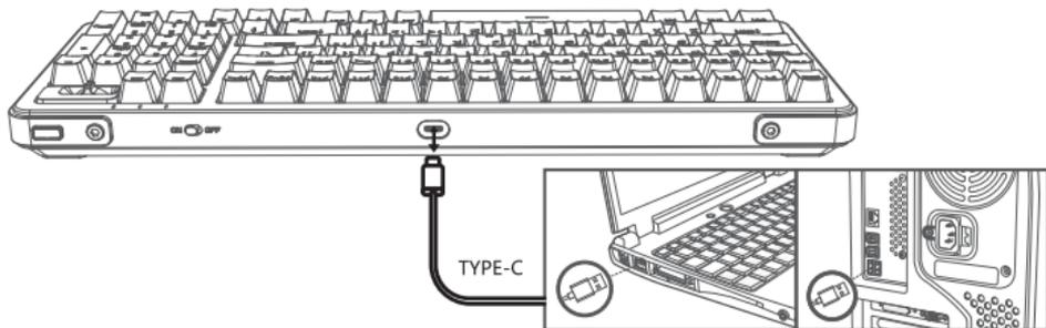
2. Plug the charging cable' TYPE-C interface into the keyboard, USB interface into your computer to start charging,
